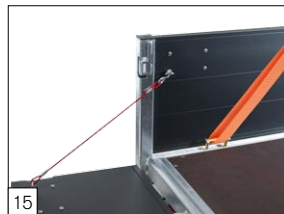
Standard: TÜV certified HAPERT load-securing system. These binding brackets are integrated in the sides with a capacity of 1000 daN each.
