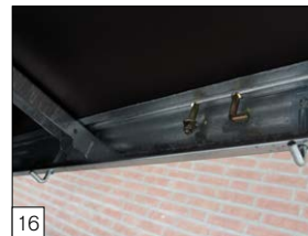
Option: boltable rope hooks mounted underneath the sides edges.
