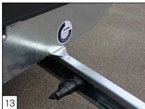
Standard: resistance unit for the LED-lighting.
