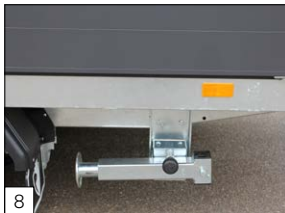
Standard: the prop stands are adjustable and 90° swivelling.
