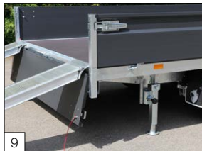
Standard: U-profile at the rear to put on the loading skids.
