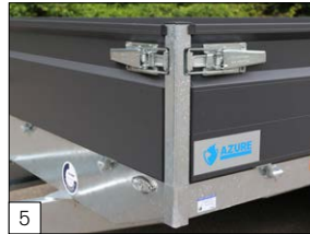
Standard: aluminium dropsides 40 cm high with a coating in anthracite.
