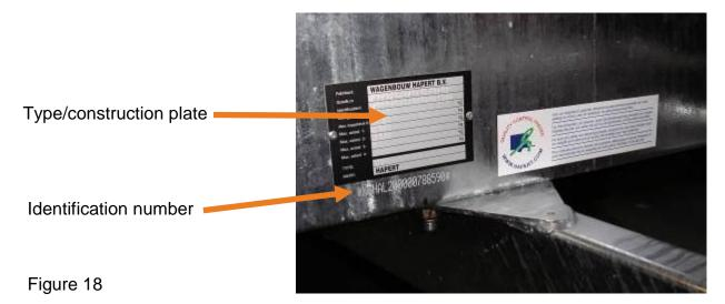
Location of the type plate of an ECE-approved tow pole: against the tow pole For trailers with a pipe tow shaft, it is located on the shaft. (See figure 19)
