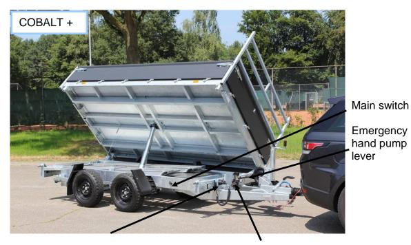
Electric operation switch Emergency hand pump valve
