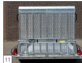
**Standard:** continuous tail ramp with a height of 1500 mm, including supports and high-quality suspension.
