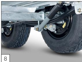
**Option:** parabolic suspension including shock absorbers.
