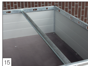
Option: load-restraint tubing mounted.
