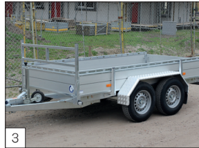
Option: mudguards made of aluminium tread plate.
