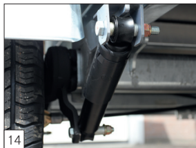
Option: shock absorbers mounted on axles.
