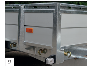
Option: boltable hooks on the outside.
