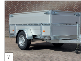
Option: removable aluminium walls with a height of approx. 40 cm, provided with durable locks.
