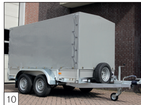
Option: raised cover mounted and spare wheel with support in front.
