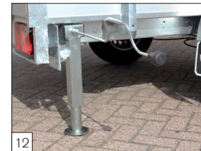
Option: adjustable, swivelling, telescoping prop stands and provided with removable crank.
