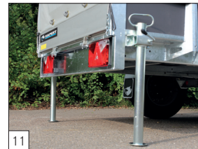
Option: sliding prop stands mounted with clamping bracket.
