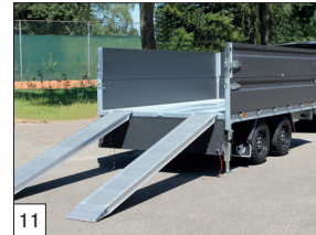
Standard: "drive-on" kit mounted (2 loading skids and prop stands).
