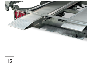
Standard: 2 aluminium loading skids 2500 mm. long integrated underneath the floor.
