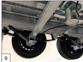
Standard: parabolic leaf spring axles incl. shock absorbers.
