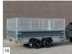
Option: a weldmesh side extension 75 cm high on all sides and a pendulating backwall.
