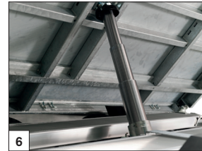
Standard: a built-in, solid, hydraulic 5-steps cylinder and a "FERRO"-floor kit: a single hot dipped, galvanised 3mm thick steel plate.
