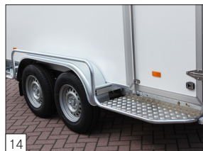
Option: protective brackets on the sides, provided with aluminium foot plate.
