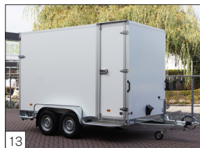
Option: side door has been provided with stainless steel locks and hinges.
