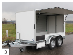
Option: side hatch and small hatch in front of the mudguard, hinged downward.
