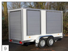
Option: aluminium rolling hatch on the rear and sliding hatches on both sides.
