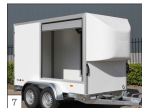
Option: aluminium sliding hatch in side wall.
