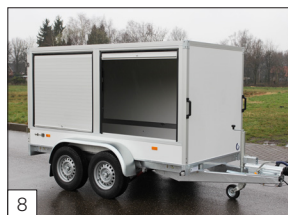
Option: 2 aluminium sliding hatches (maximum width 150 cm) in the side wall, including centre post.
