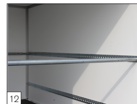
Option: load-securing system inside the closed superstructure, provided with load-restraint tubing and securing strap.
