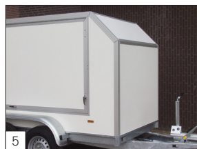
Option: bevelled front (identical angle approx. 40 x 40 cm).
