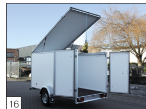
Option: lid hinged on the front (possible with maximum dimensions of up to 300 x 150 x 180 cm).
