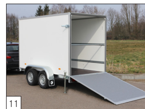
Option: tail ramp provided with grey antiskid coating.
