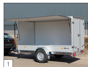
Option: side hatch mounted, opening either to the left or to the right (in driving direction).
