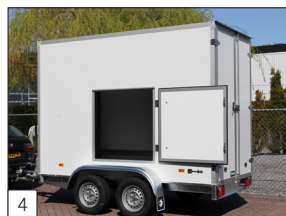
Option: small hatch in side wall.
