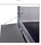
The H models have a U-profile at the rear. They also come prepared for the later addition of a storage compartment with drive-on ramps under the floor (with the exception of model H 260 x 150 cm).
