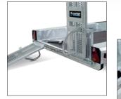
The rear of the LF models has a drive-on ramp in one piece of approx. 1500 mm with brackets. Optionally available: two steel drive-on ramps. These ramps are width-adjustable. The ramps consist of an open anti-slip grating profile and are full-immersion galvanised.
