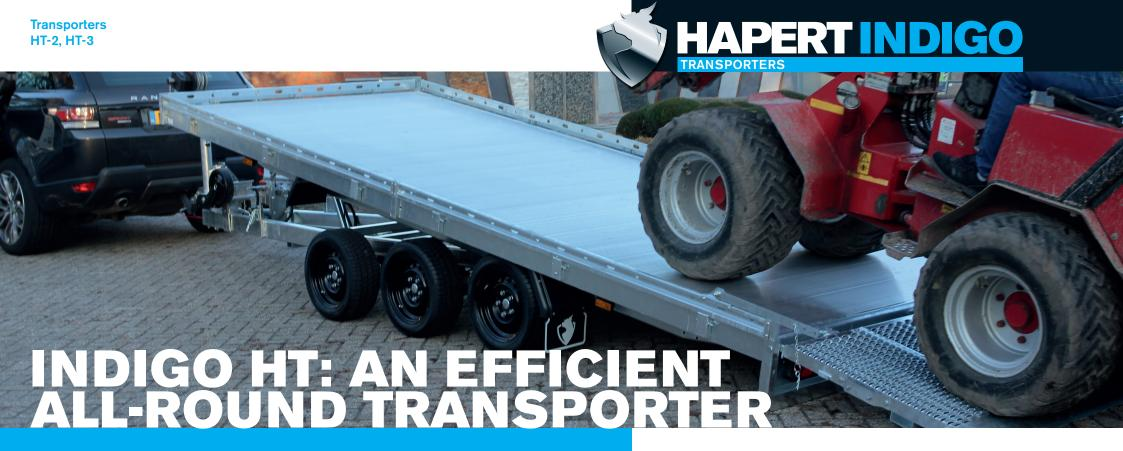
The Indigo HT is a solid tiltable transporter. Thanks in part to its 100-cm continuous tailgate and the double-acting hydraulic system, it's flexible and can quickly be prepared to transport 3 or 4-wheel machines and other vehicles.
