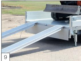
**Option:** DRIVE-ON kit mounted: 2 aluminium loading skids 250 cm long, 2x 90° swivelling heavy duty prop stands and support crank.
