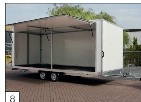
**Option:** large-sized side hatch with centre post in place.
