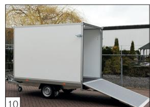
**Option:** tail ramp provided with grey antiskid coating. Ramp provided with gas springs.
