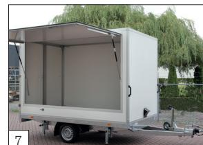
**Option:** side hatch with bottom part of the side wall fixed and 4 prop stands mounted.
