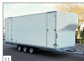
**Option:** three-axle version with 2 side doors (front and rear) and spoiler.
