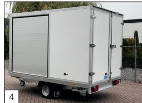
**Option:** aluminium sliding hatch (max. dimensions: height 180 cm x width 150 cm) in the side wall.
