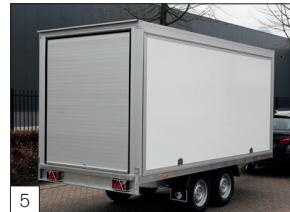
**Option:** aluminium sliding hatch on the rear, and rear-light protection.
