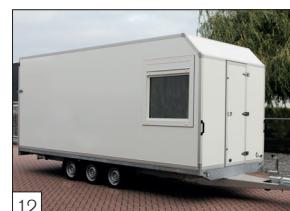
**Option:** three-axle version with window and bevelled front (angle approx. 40 x 40 cm).
