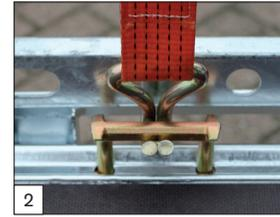
**Standard:** with TÜV certified load securing system with 1000 daN (Kg) for each fixing point.
