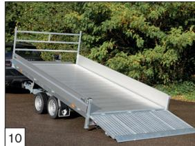
**Option:** aluminium dropsides 300mm and a ladderrack in front. (a ladderrack is only possible in combination with dropsides).
