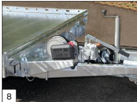
**Standard:** a multi-adjustable winch with support mounted in front.
