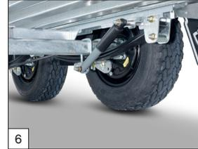
Parabolic leaf spring axles incl. shock absorbers (parabolic axles not possible for models in 405 cm).
