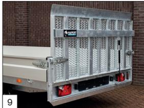
**Standard:** a tailramp 100 cm high including a gas spring and heavy duty fasteners.
