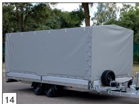
**Option:** high cover in 180 or 210 cm high and the frame construction is removable and modular.
