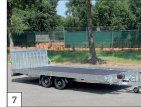
**Standard:** tyres 195/50 R13 C with black rims for the models in 450 and 505 cm with parabolic leaf spring axles.
