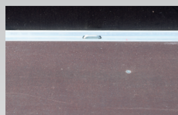
Multiplex floor 12 mm provided with an anti-slip layer
