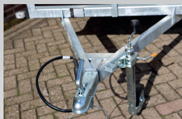
Bolted V-drawbar 105 cm long incl. breakaway cable
