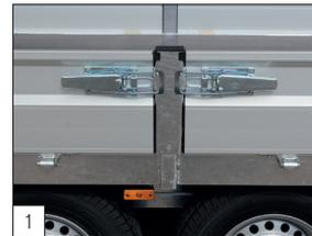
**Standard:** the H models with a length of more than 450 cm are, as a standard, equipped with removable central posts.
