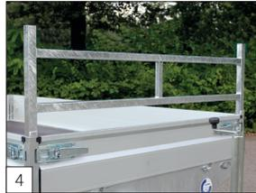
**Option:** removable front rack mounted and secured in the corner posts.
