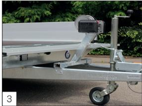
**Option:** winch and winch support mounted in front (only possible in combination with walls with a height of 30 cm).
