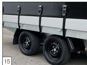
**Option:** for all the Azure H models with parabolic leaf spring axles the tyres 185 R14C, 185/70 R13C and 195/50 R 13 are with black rims.
