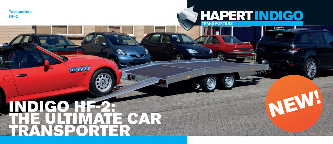
This new trailer has been specially developed for the transport of all kinds of cars. The Indigo HF-2 is therefore available in three sizes: 405 x 201 cm & 455 x 201 cm & 505 x 221 cm. and in different loading capacities. The car transporter is even available with parabolic suspension.
