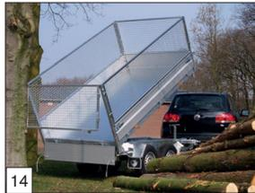
**Option:** removable wire-mesh rack with a height of 70 cm and wire-mesh racks with a height from 335 cm upward, reinforced with side posts.
