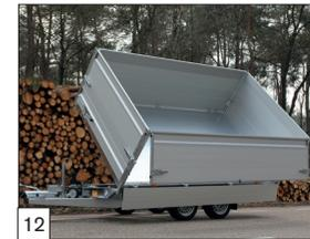
**Option:** aluminium drop-sides with a height of 70 cm, pendulating.
