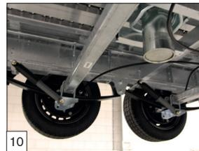
**Option:** parabolic leaf spring including shock absorbers on the axles.
