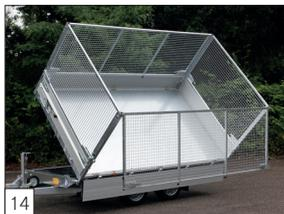
**Option:** a weldmesh side extension on all sides, removable, height 75 cm (extensions are reinforced).
