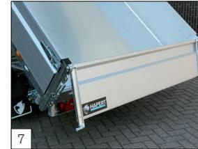
**Option:** a pendulating rear dropside (only possible in combination with dropsides 40 cm).
