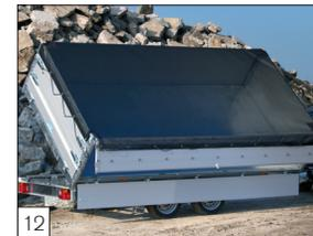
**Option:** removable, pendulating aluminium dropsides 40 cm high including a cargo net.
