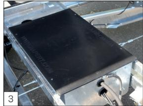
**As standard:** electric control powered by a battery enclosed in a steel box.
