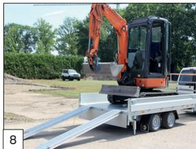
**Option:** 'DRIVE-ON' package: 2 aluminium loading skids integrated underneath the floor and 2 stable, adjustable telescoping legs including crank.
