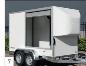
**Option:** aluminium sliding hatch in side wall.
