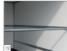
**Option:** load-securing system inside the closed superstructure, provided with load-restraint tubing and securing strap.
