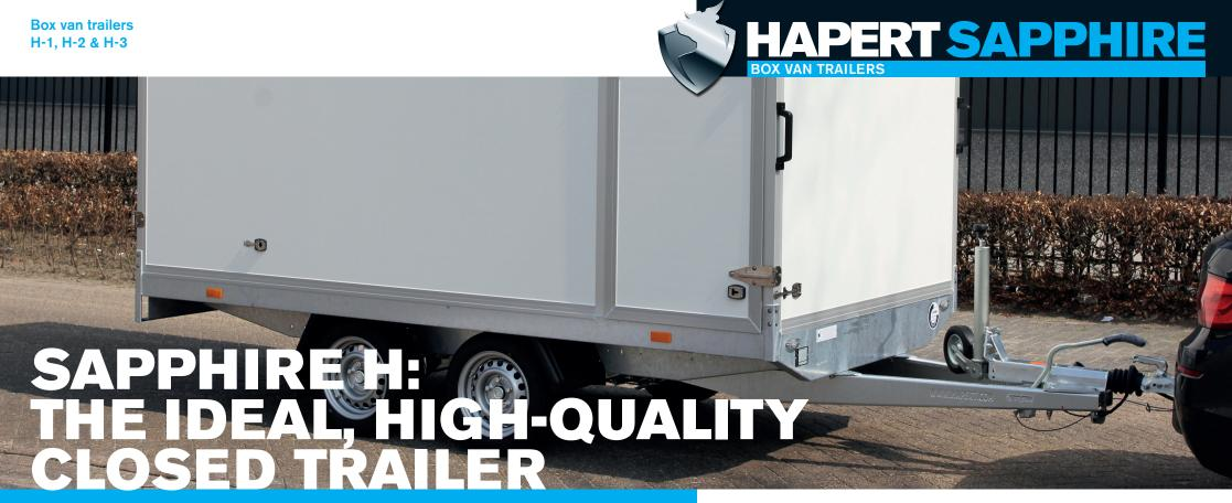
Thanks to the welded, hot-dipped galvanised substructure as well as the incredibly strong superstructure, the Sapphire H models are eminently suitable to transport your valuable cargo from A to B without any problem.
