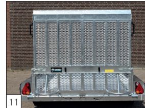
Standard: continuous tail ramp with a height of 1500 mm, including supports and high-quality suspension.
