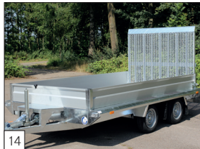
Option: aluminium front and side boards with a height of 30 cm.
