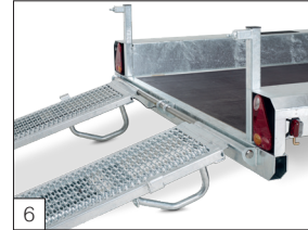
Option: 2 steel galvanised loading skids with a length of 150 or 200 cm, hinged at the back.
